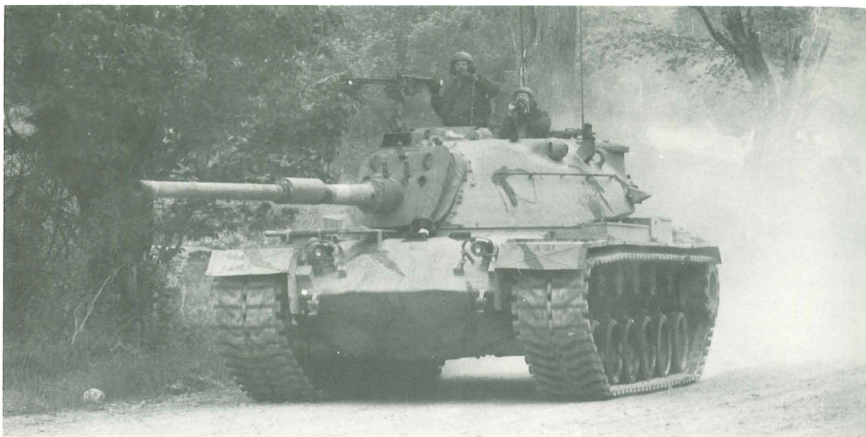
An M48A5 of the 50th Armd. Div. (National Guard) during summer manoeuvres at Camp Drum, NY in 1980. This vehicle is an M48A5 (Low Profile) with the Urdan commander's cupola and twin M60 pintle-mounted machine guns on the roof. (Midic Castelletti)
