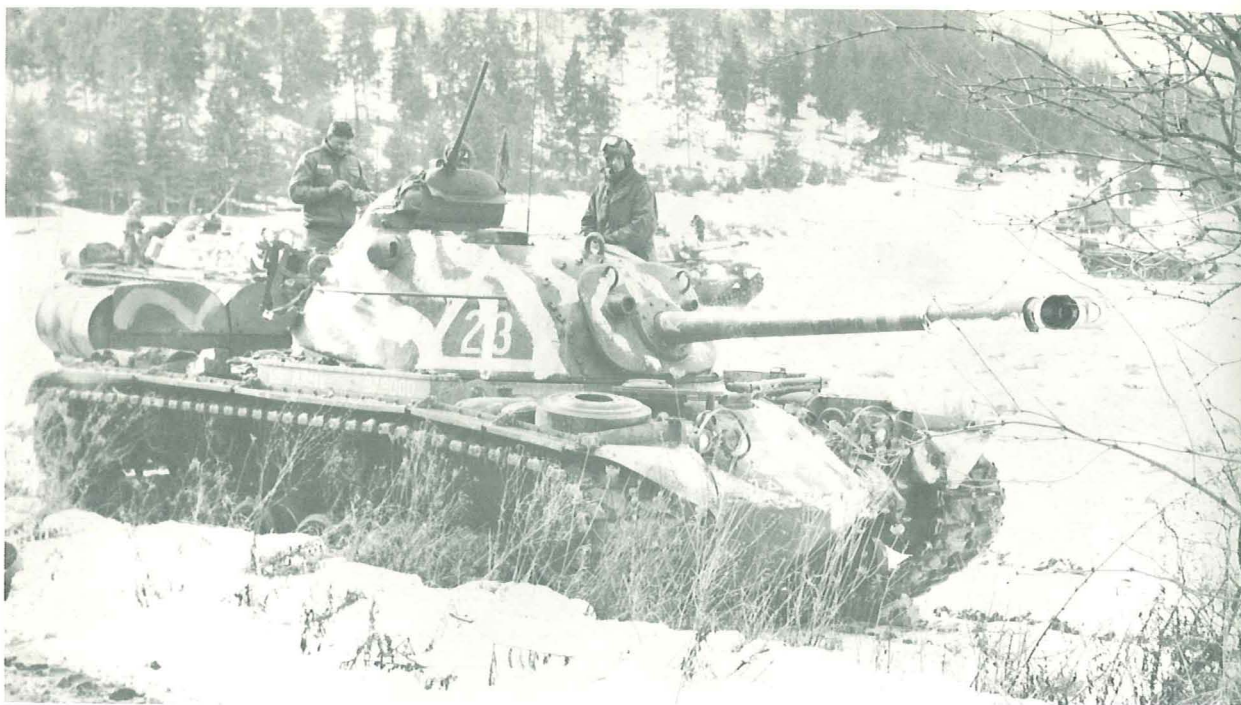
An M48A1 of 37th Armor, 4th Armd. Div. takes part in Exercise 'Wintershield II' near Allersberg, Germany on 3 February 1961. The M48A1 was the first tank of the series to be fitted with the distinctive M1 commander's cupola. This particular tank is fitted with the Universal Jettison Fuel Tank Kit on the rear to extend its effective range. (US Army)
