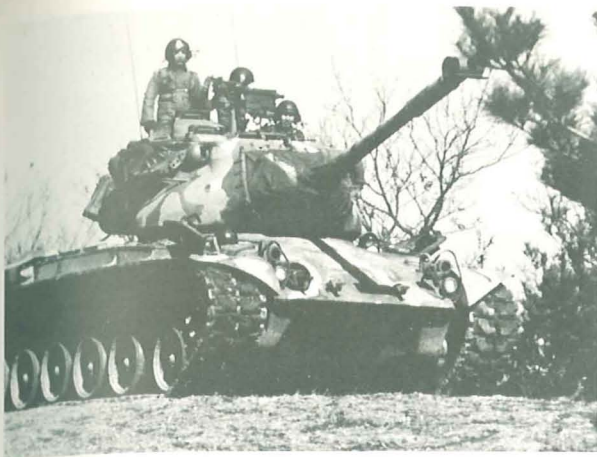
This Korean M47 is from the later production batches fitted with a T-shaped muzzle brake. (George Balin)
