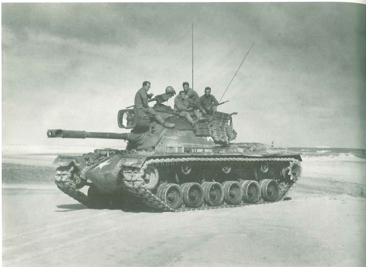
An M48A3 of 'M' Co., 3rd Sqn., 11th Cavalry churns forward during Operation 'Junction City' near Lai Khe, Vietnam, 13 April 1967. The M48A3 (Late Model) was the preferred Patton, since—unlike this vehicle—it was equipped with a G305 cupola vision riser which gave the commander better all-round vision. (US Army)
