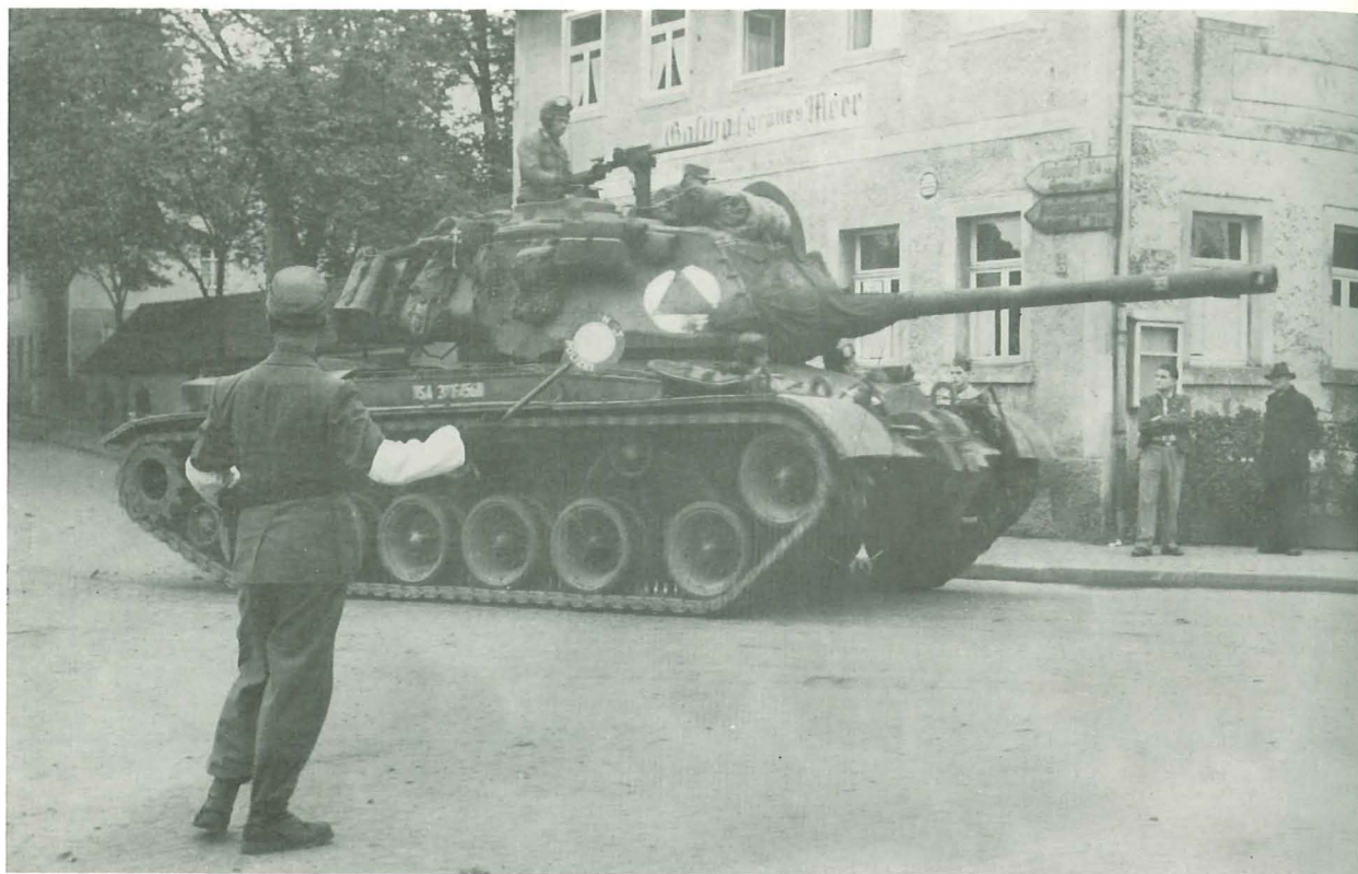
An M47 Patton of the 12th Regimental Combat Team advances through Dinkelsbühl, Germany on 13 October 1955 during Exercise 'Cordon Bleu'. This is an early production vehicle with the initial turret grab-irons. The green-triangle-on-white-circle insignia is the traditional manoeuvre marking for 'aggressor' forces. (US Army)
