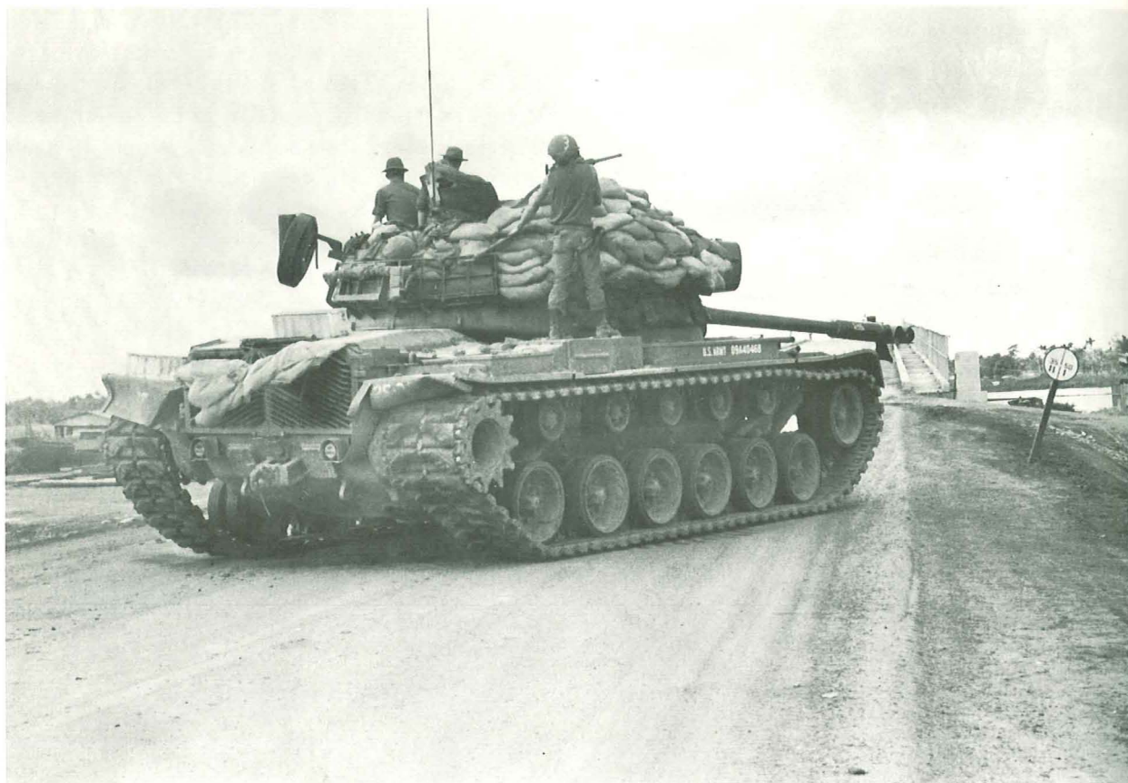
Pattons were frequently used for convoy duty in Vietnam. After this vehicle was hit by RPG-7s with some crew casualties, the rest of the crew erected a sand-bag parapet around the turret roof to offer better protection against close-range grenade attacks. This M48A3 served with 3/4th Cavalry supporting the 25th Inf. Div. in July 1968. (Col. James Loop)
