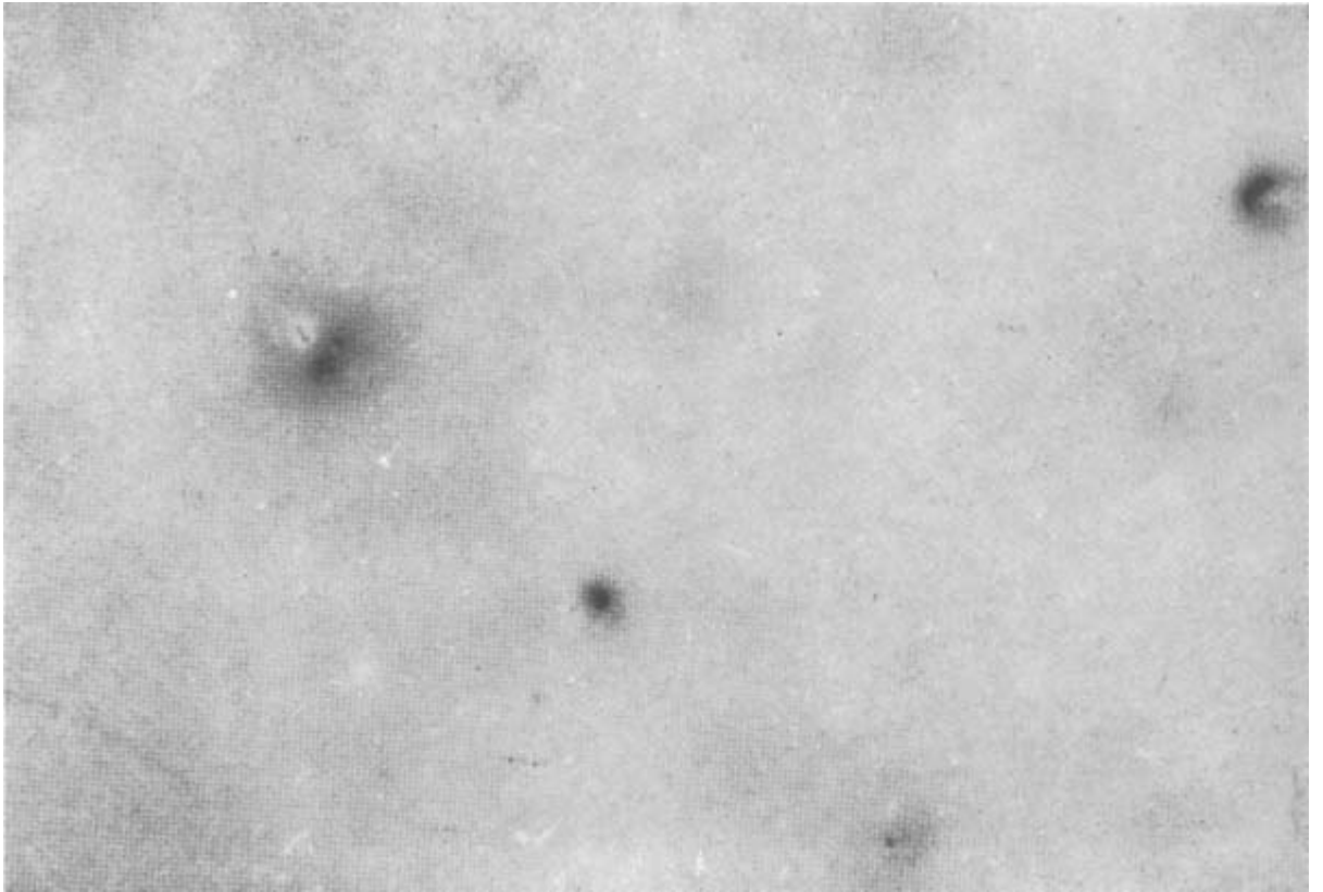
Figure 43 Gelcoat fault - fish eyes
