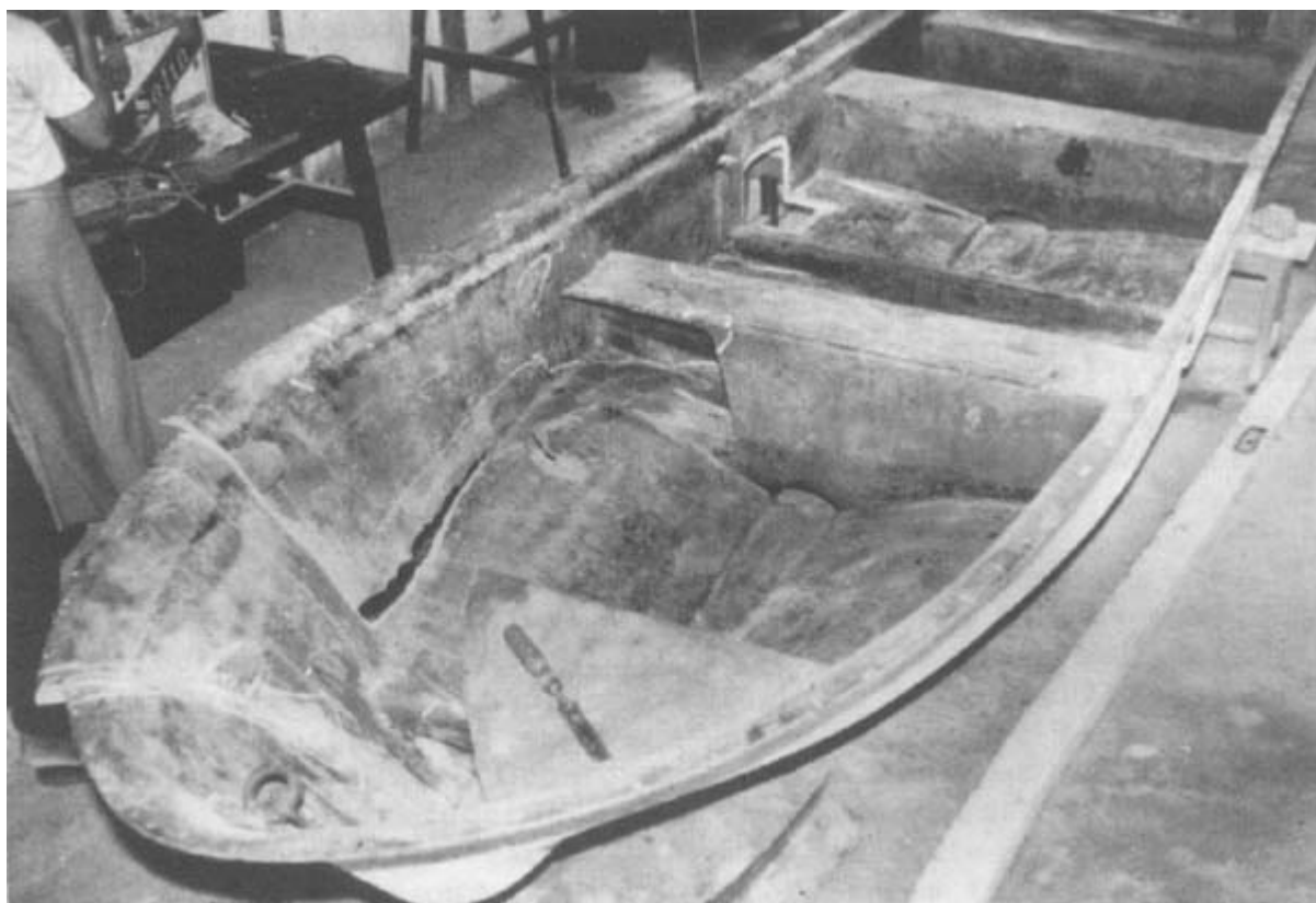
Figure 55 Severe impact damage to side
