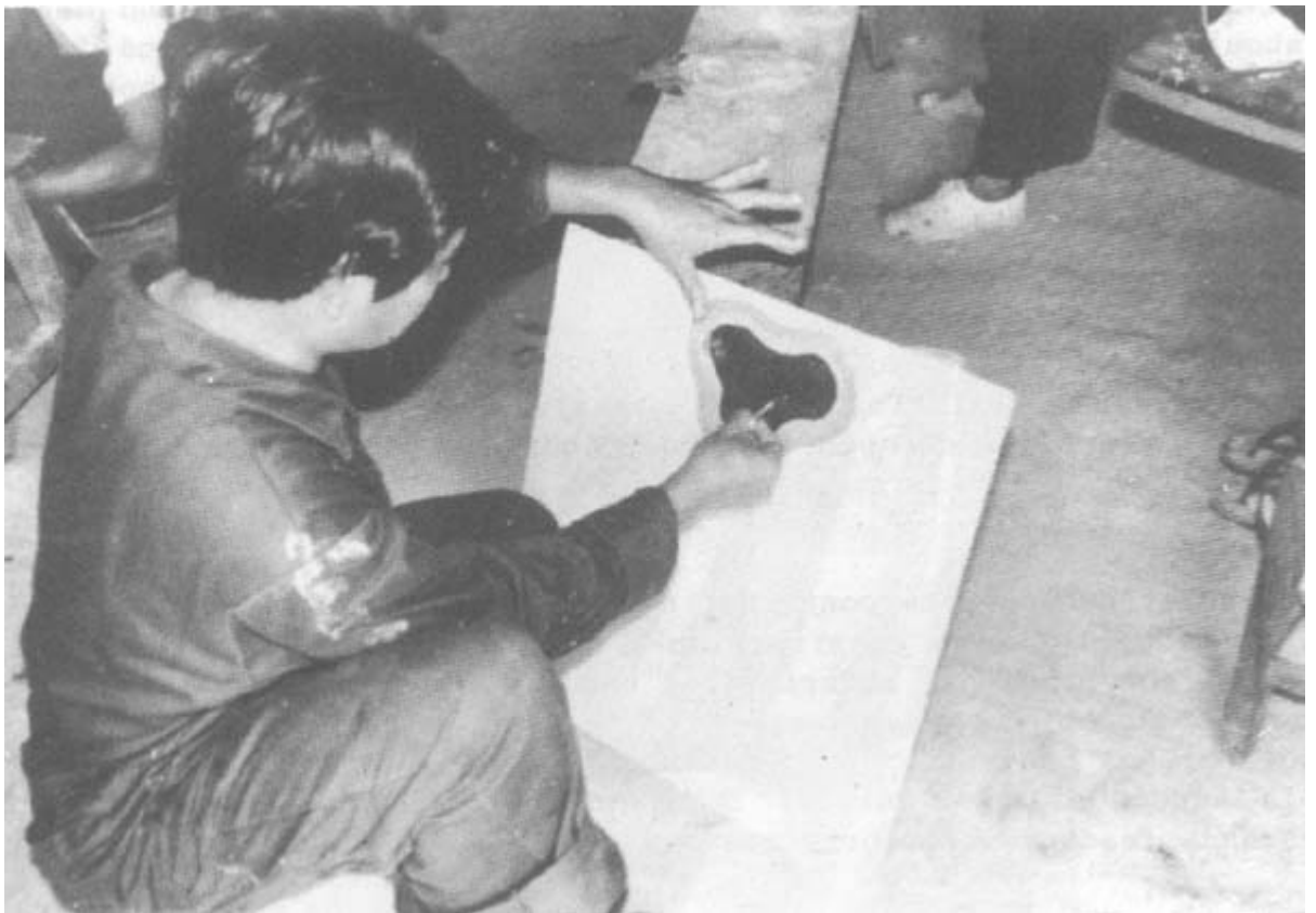
Figure 25 Repairing one-side access hole
