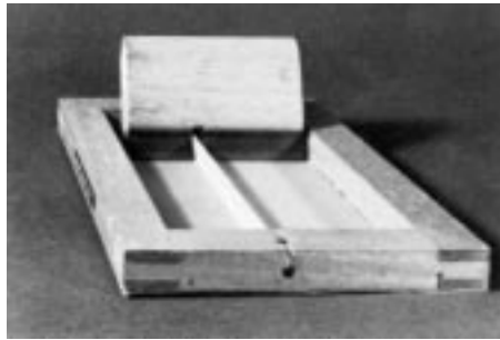
Split stencil for two-color printing
