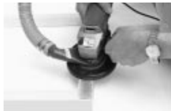
Rotary grinder with integrated dust extractor
