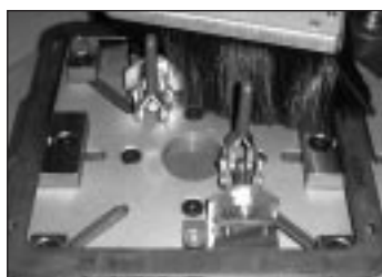
Sefar America SBM-400 CD frame stripper.
