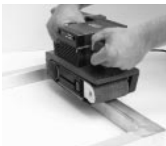
Belt sander, no. 24–36 grit. This technique gives a flatter frame.
