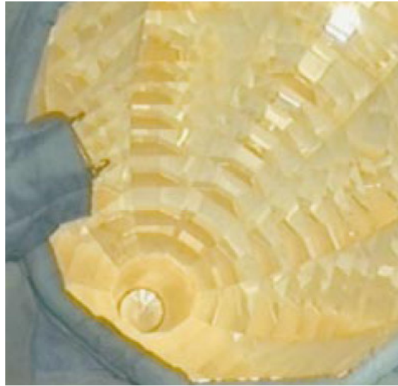
Fig. 2-23 Secondary concentrator (CPC) at the Weizmann's Institute solar power tower /SolarPaces 2001/
