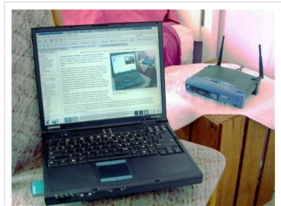
This notebook computer is connected to a wireless access point using a PC card wireless card.
