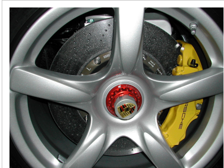
The Porsche Carrera GT's carbon-ceramic (silicon carbide) composite disc brake
