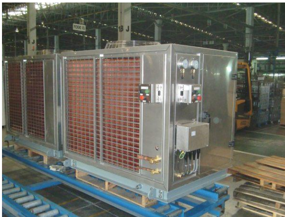
38 kW Air Cooled Condensing Units Chim Sao PTSC Vietnam
