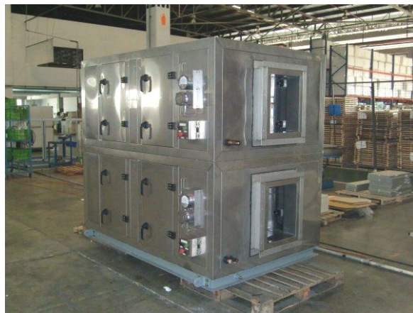
38kW Double Stacked AHU Chim Sao PTSC Vietnam
