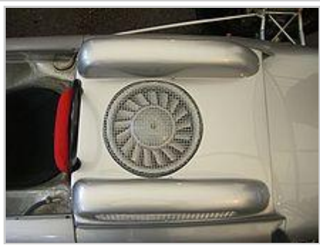
Porsche 804 had a cooling fan to cool the air-cooled flat-8 engine.
