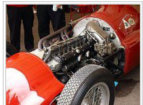
This Alfa Romeo 159 supercharged straight-8 engine of 1950s could produce up to 425 bhp.
