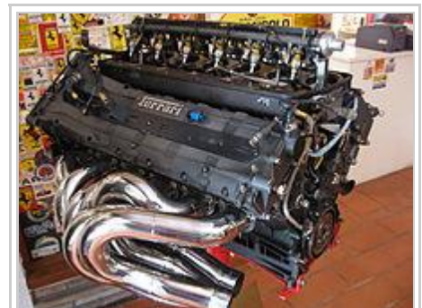
This Ferrari 3.0 litre V12 F1 engine (1995) produced 700 hp (522 kW) at 17,000 rpm
