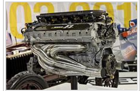
A 1990 Renault RS2 V10 engine.
