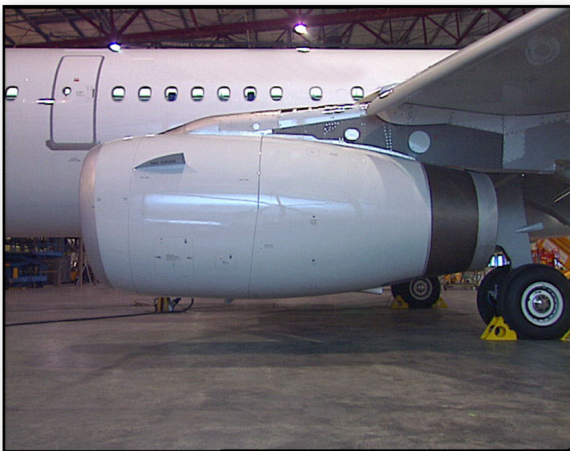
THRUST REVERSERS STOWED -TRANSLATING SLEEVE CLOSED-
