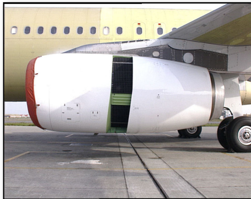
THRUST REVERSERS DEPLOYED -TRANSLATING SLEEVE OPEN-
