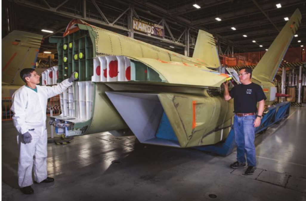
Northrop Grumman has delivered the centerbody/aft fuselage for the first RAAF EA-18G to the Boeing final-assembly facility in St. Louis. The section, which was the 115th Growler subassembly completed at Northrop Grumman, is the first of 12 destined for Australia.
