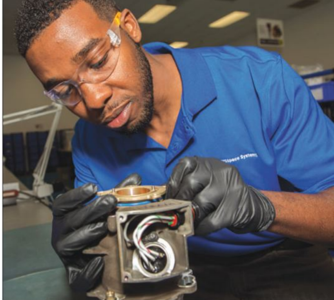
A repair technician at UTC Aerospace Systems works on a boost pump at its Miramar MRO facility.
