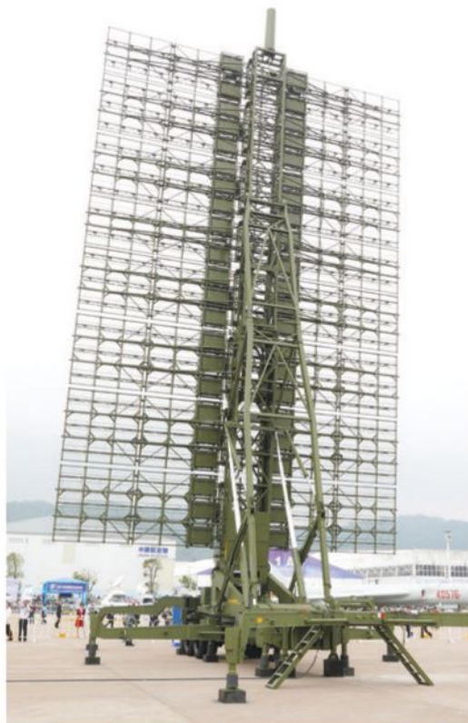
The CETC JY-27A Skywatch-V, China's first VHF AESA, is in production for Chinese air defense units.
