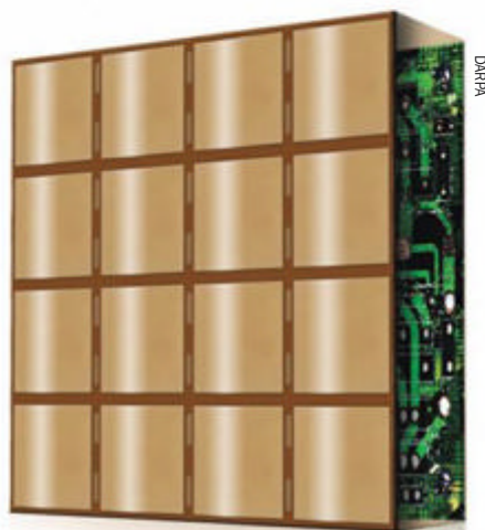
ACT common module mounts directly to array to provide digital beam-forming at each element.
