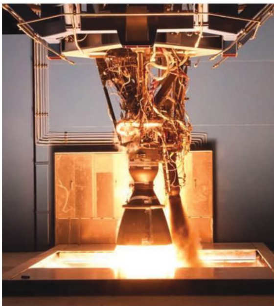
An upgrade to the SpaceX Falcon 9 Merlin 1D engine aims to increase thrust by 15%.
