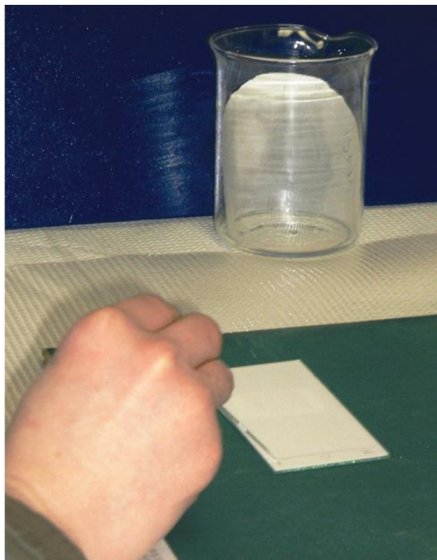
Figure 4.13 A thin layer chromatography set-up. The filter paper in the beaker is there to keep the atmosphere inside the container saturated with mobile phase. This can greatly improve the quality and reproducibility of the chromatogram.
