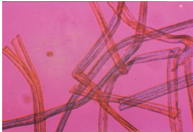
Figure 6.14 White acrylic fibers under polarized light. The orange and blue interference colors are due to the different interactions of the fibers owing to their orientation toward the polarized light.
