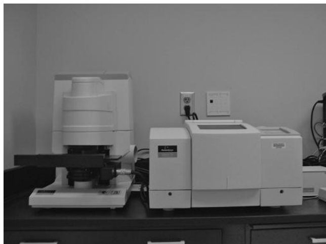
Figure 6.17 An infrared microspectrophotometer. The infrared spectrophotometer is on the right side of the picture. This is connected by a light pipe to the microscope on the left. The infrared light travels from the bench, through the microscope and then to a detector mounted inside the microscope. There is no ocular lens. Instead, a video camera captures the images and sends them to a computer. The stage is controlled by a joystick.
