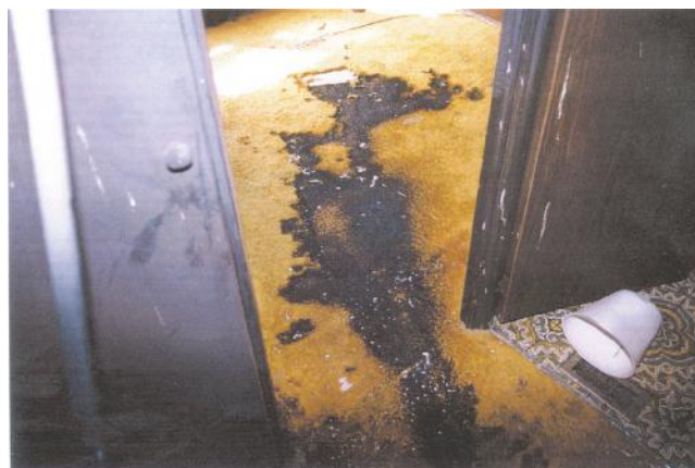
Figure 20.5 A fire trail in a mobile home. Courtesy of Charles Hughes.
