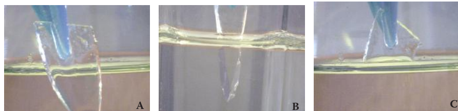
Figure 19.14 A shows a small piece of Pyrex glass not immersed in a liquid. B shows the same piece of glass immersed in water. C shows the piece immersed in vegetable oil. Pyrex and vegetable oil have similar indices of refraction as evidenced by the disappearance of the glass in the oil.
