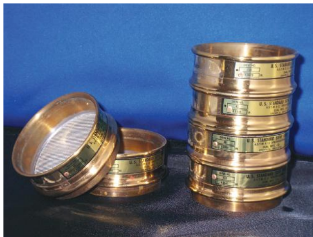
Figure 4.2 A group of nested sieves. Each sieve has a finer mesh than the one above it. The sieves are put in a series and soil or other material is poured through it. After gentle shaking, the soil is distributed throughout the sieves by particle size.
