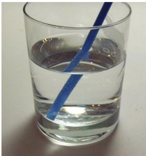
Figure 19.10 Refraction of a plastic straw partially immersed in water. The straw appears to bend because of refraction.
