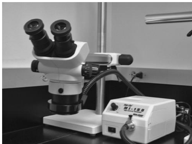
Figure 6.9 A stereo microscope. Note the absence of a stage. Specimens are mounted directly on the table. Light is supplied by a light ring below the objective lens.
