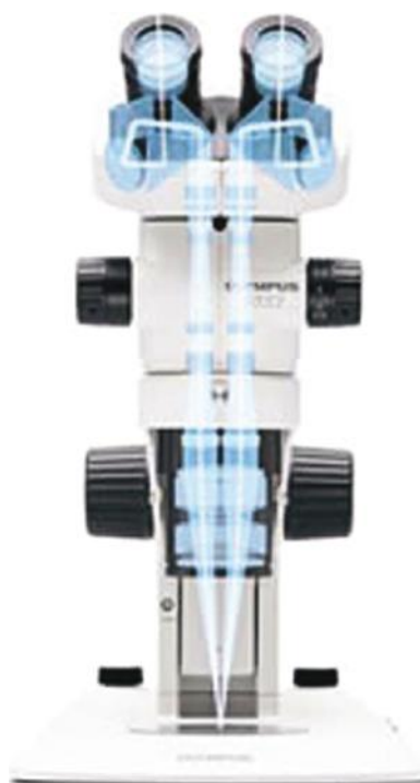
Figure 6.10 The light path through a stereo microscope. Note that the two light paths converge slightly away from each other, thus creating the three-dimensional image.
