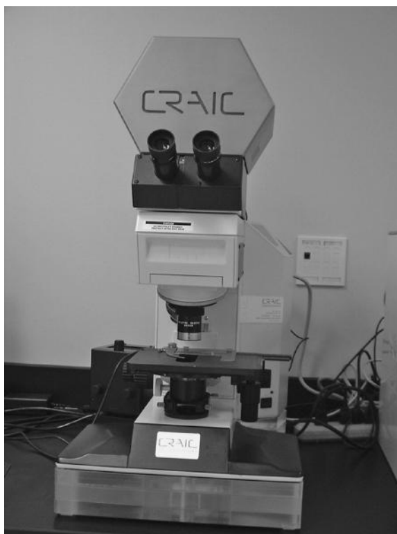
Figure 6.15 A microspectrophotometer. The large box on top of the microscope is the detector. Ultraviolet, visible, and near infrared light can be used as the light source.
