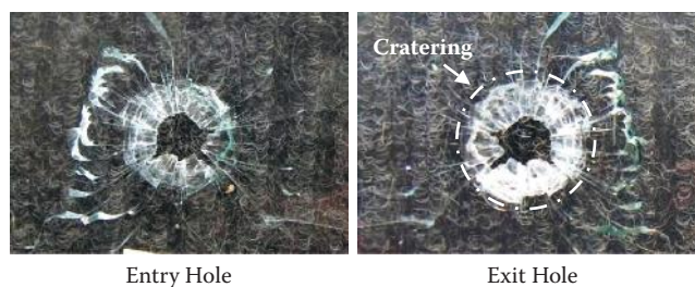
Figure 19.5 Entry and exit holes produced by the same bullet going through a glass window. The hole on the left is entry, characterized by a smoother hole and no cratering on the entry side. The hole on the right is exit, characterized by the cratering around the entry hole (whiter areas around the hole highlighted by the dotted circle).
