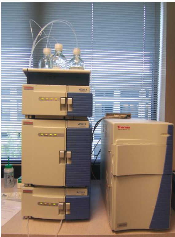
Figure 4.12 A photograph of an HPLC instrument. These instruments are generally quite modular so that a variety of pumps can be mounted into the system. There is also room for several detectors mounted in series.
