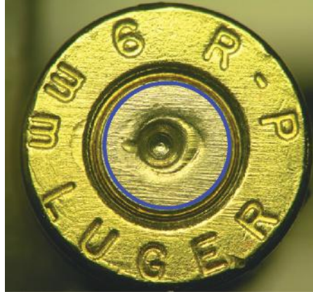
Figure 9.12 The nickel center of this cartridge case is the primer cup (shown circled). The firing pin strikes this part of the cartridge in the gun chamber to initiate the explosion. Courtesy of www.precisionforensictesting.com .
