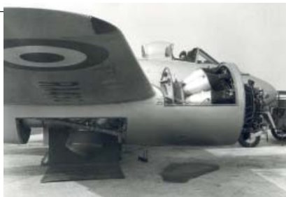
The vectored thrust Meteor jet fighter demonstrator preparing to ground run at Yeovil showing the Nene engine placed ahead of the wing and the deflector jet pipe.
