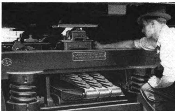
Fig. 7—Leaf and coil springs on New York Central “Mercury”
