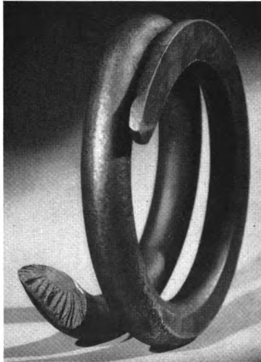
Fig. 25—Typical fatigue failure
