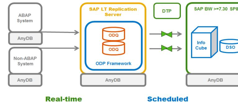
**Option 3:** Setup with Data Transfer Process into BW Data Targets and RDA Daemon possible with SAP BW 7.40 SP5
