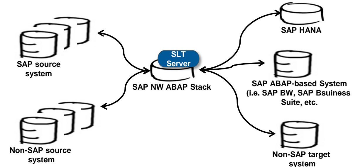
Recommendation: In order to separate workload a separate SLT Server system is the most preferable option for productive use. Especially when to expect high data transfer rates and/or to keep independent patch/release cycles.
