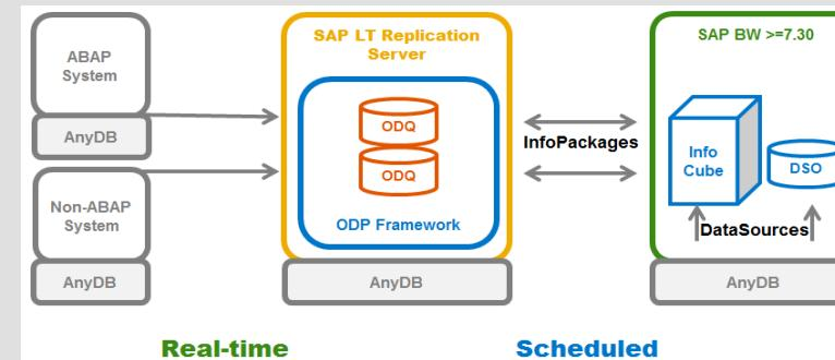
**Option 2:** Setup with Data Transfer Process into BW Data Targets possible with SAP BW >=7.30 SP8
