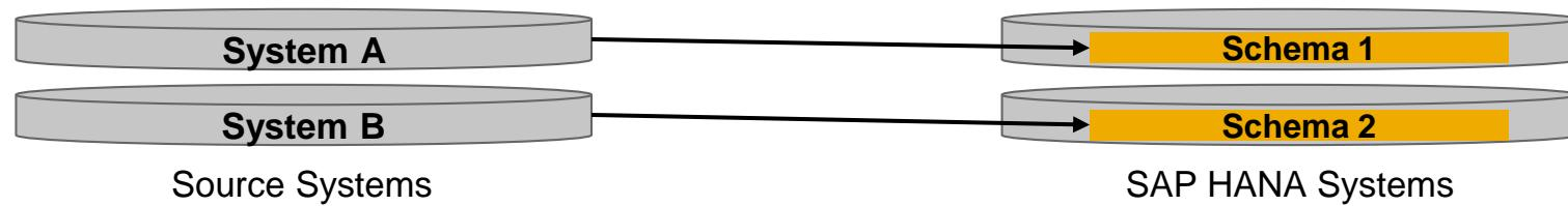
Source systems are connected to separate HANA systems. Schema name can be equal or different
