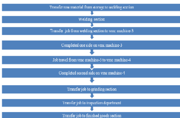
Chart 4.1 Flow process of raw material to finished stay vane
