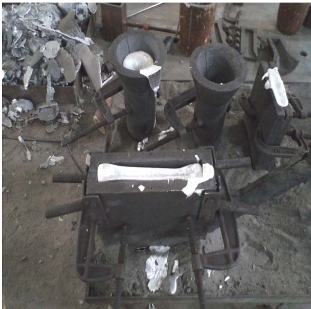
Fig. 1 Cast iron moulds allowed for solidification after the melt is poured. Moulds should be pre heated before the molten metal is poured otherwise shrinkage will occur in castings.
