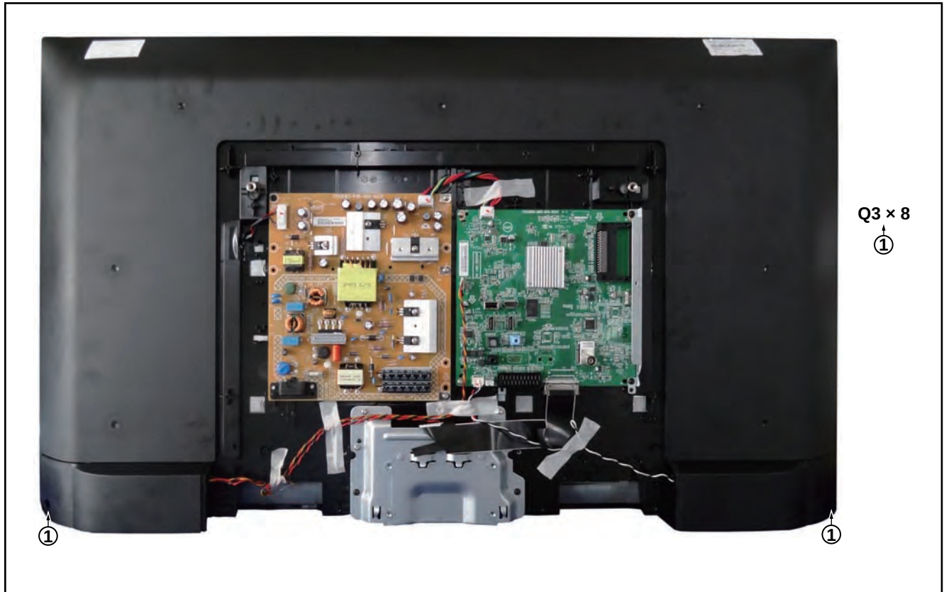
Figure 4-13 Rear cover removal [2]
