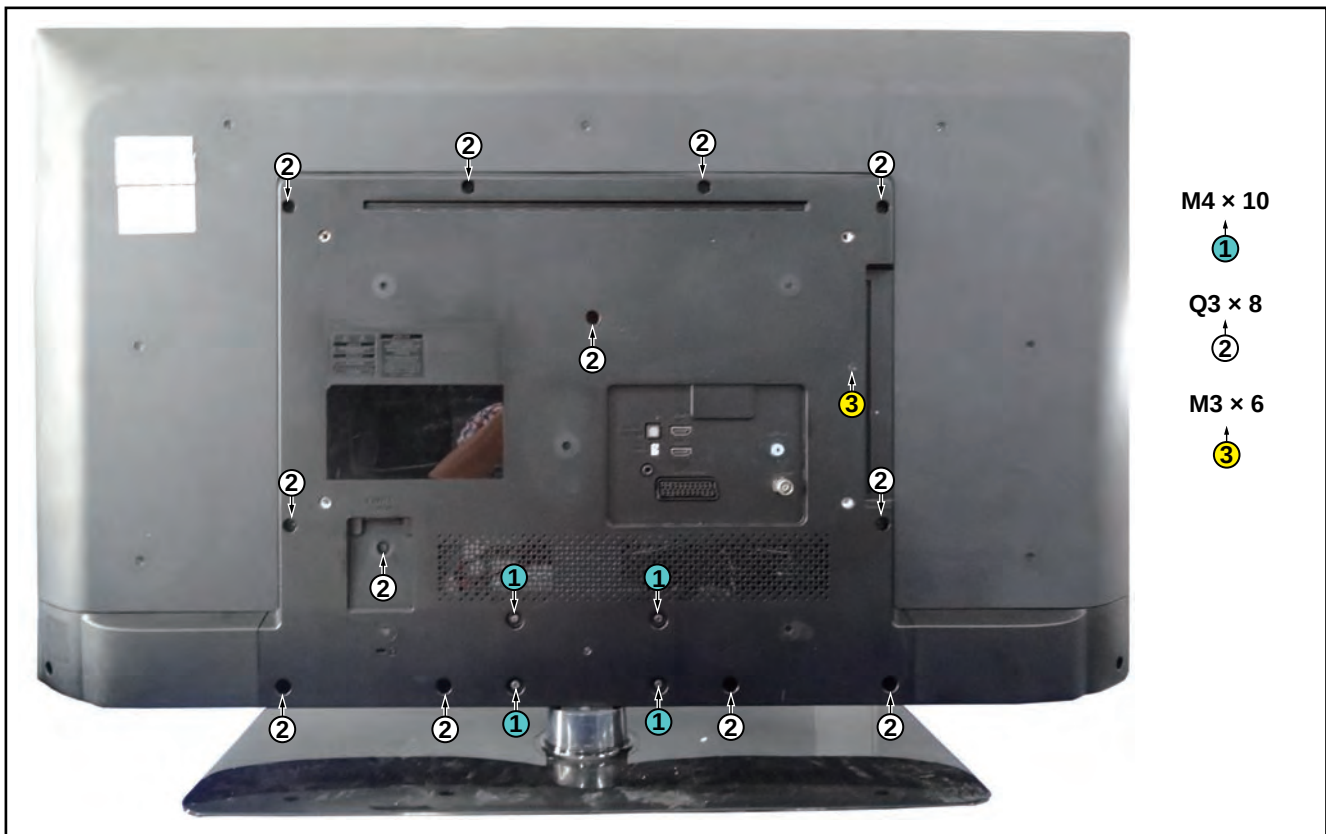
Figure 4-12 Rear cover removal [1]
