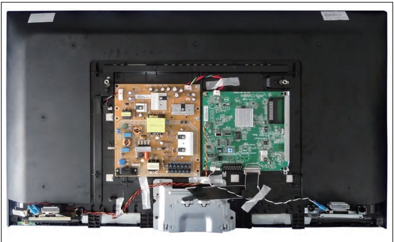
Figure 4-5 Cable dressing (40" 31x8T/60 series)
