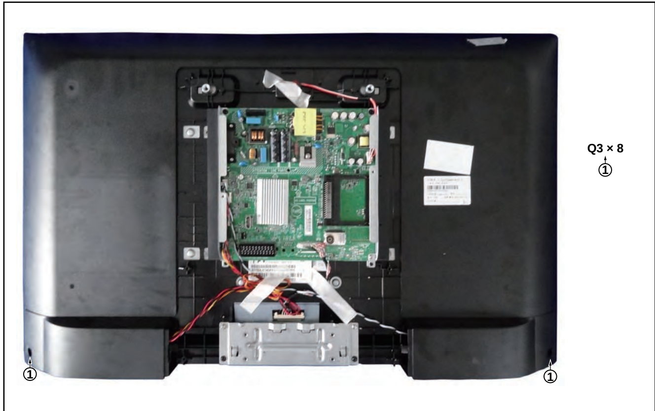
Figure 4-9 Rear cover removal [2]
