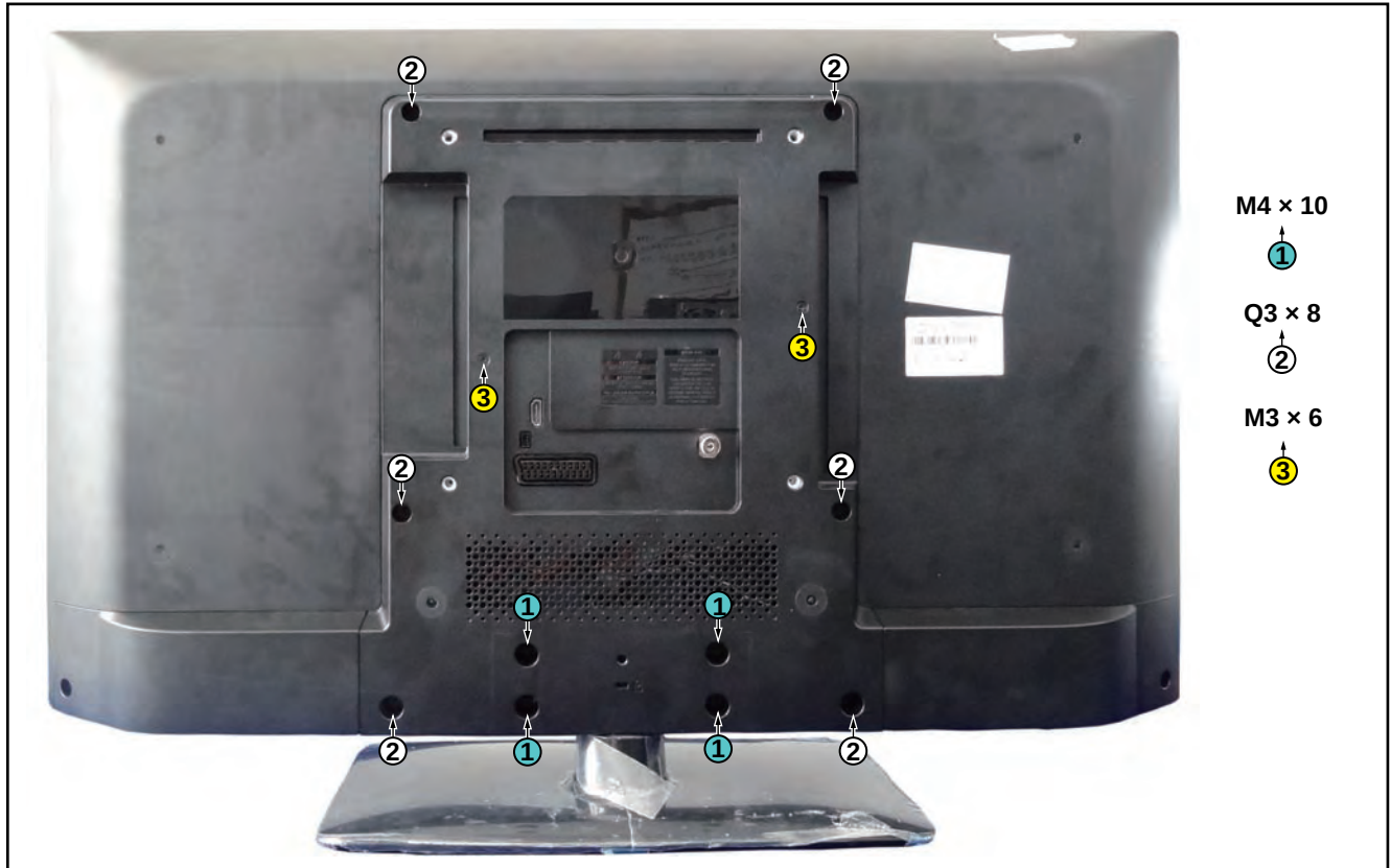
Figure 4-8 Rear cover removal [1]
