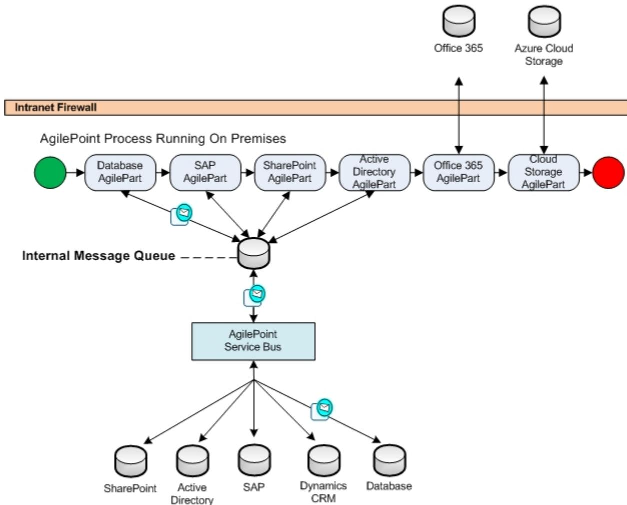
The benefit of the internal message queue is that it can move processes that take a long time out of the main processing thread, thus improving an application's **scalability**.
