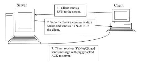
Figure 5.21 A Connection-Oriented Three-Way Handshake
