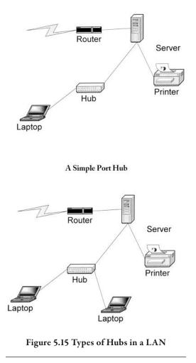
the hub passes it on in a signal form. There are two types of hubs: simple and multiple port. Figure 5.15 shows both types of hubs in a LAN.
