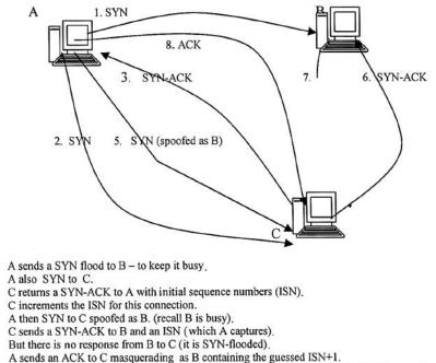
A sends an ACK to C masquerading as B containing the guessed ISN+1. If the guess is correct, then C believes A to be B and A has successfully hijacked C's session.
