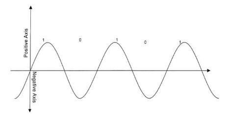
Figure 5.13 Encoding Electrical Signal and Showing of Zeros and Ones
