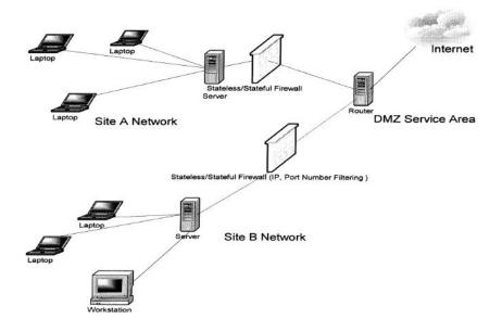
Figure 8.1 A Packet Filter Firewall
