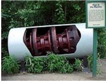
A pig in a cutaway pipeline
