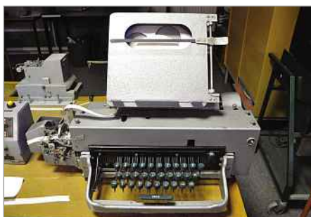
Programs for the Harwell were typed onto tape using specialised typewriters – this was the last piece to be found in storage
