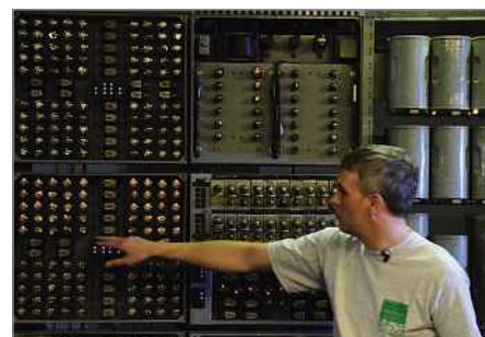
Delwyn Holroyd led the rebuild, and explained how the Dekatron valves count in decimal digits, not binary
