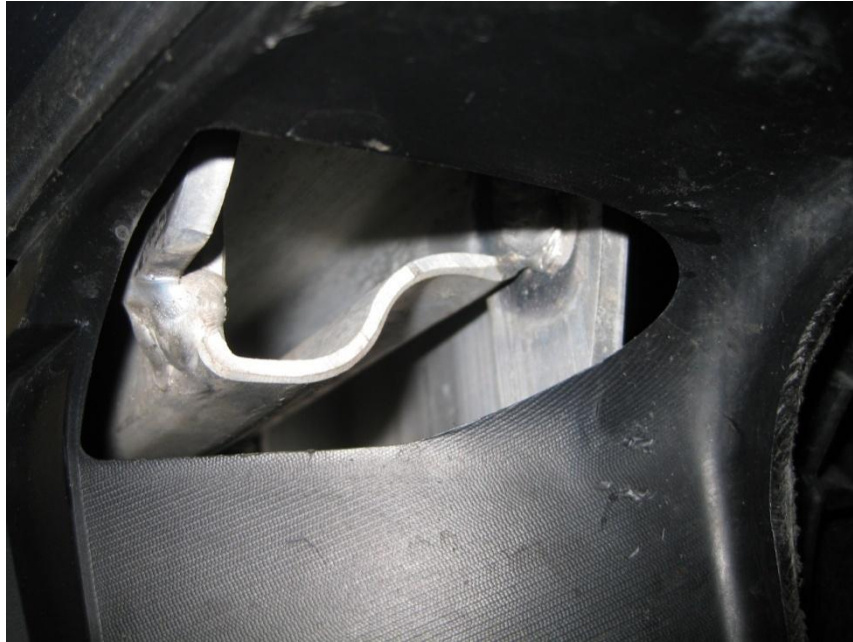
Figure 3.12: Aluminum weldments exposed after bumper trimming
