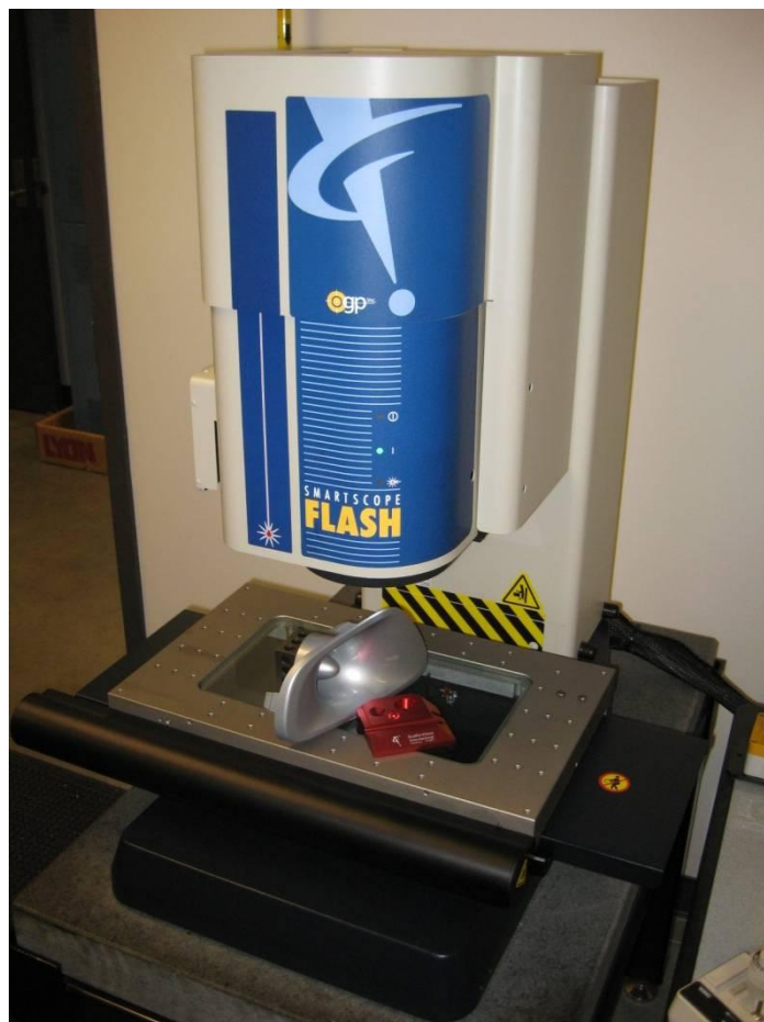
Figure 3.3: Optical measurement machine
