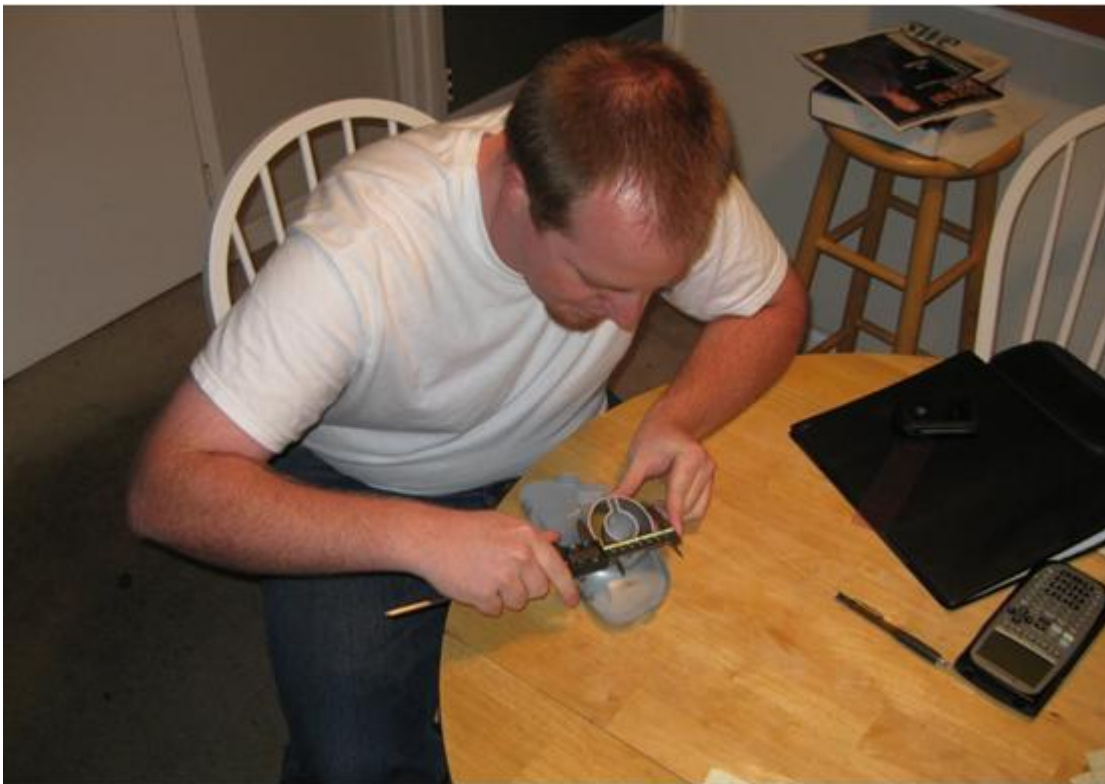
Figure 3.1: Measuring factory-installed faux duct
