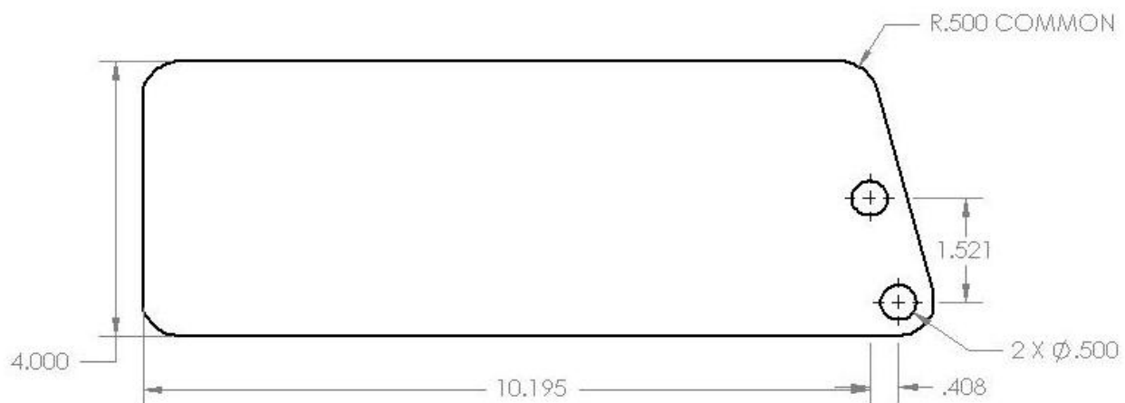
Figure 3.16: CAD Sketch of pulley bracket
