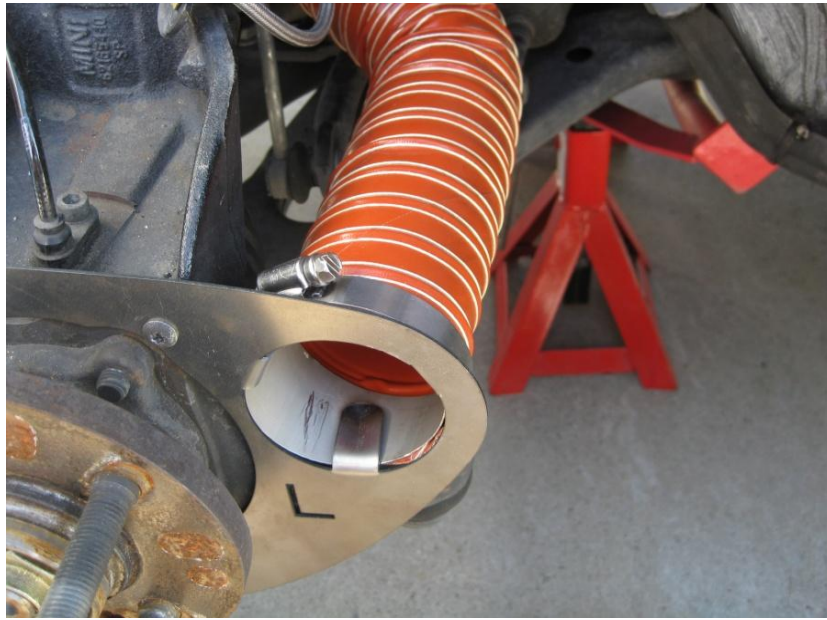
Figure A.7: Installed wheel hub bracket with attached hose
