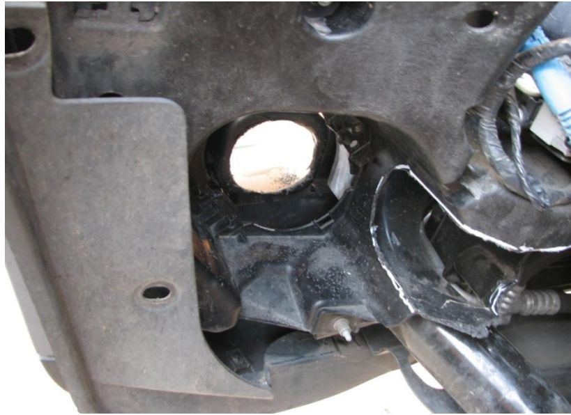
Figure A.5: Holes cut in bumper
