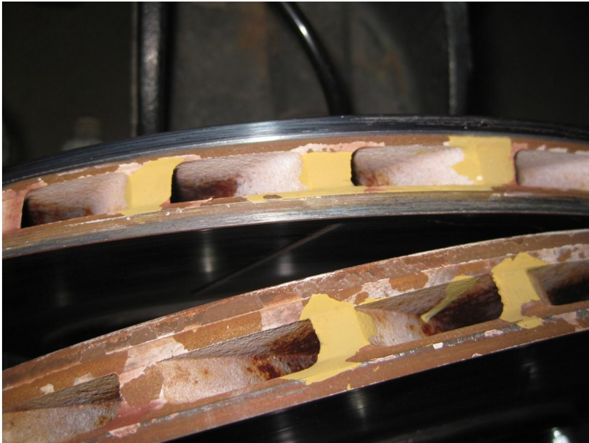
Figure 5.1: Thermal paint after testing
