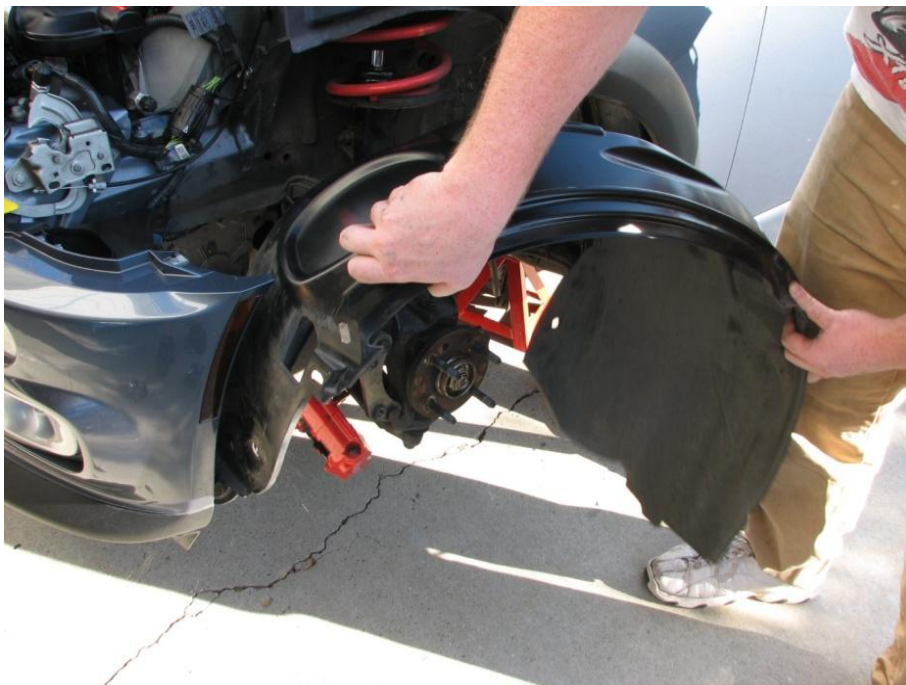
Figure A.2: Removal of wheel wells from car
