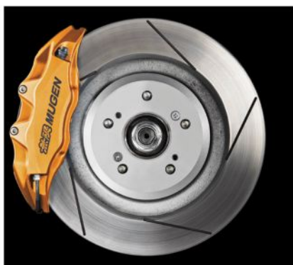
► Determining your car's bolt pattern is easy. Expressed as two figures, the first number represents the number of lugs present while the second the distance between any two non-adjacent ones.
