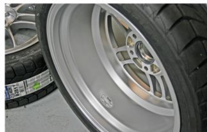
► Hub-centric wheels are manufactured with recessed centerbores that position the wheel squarely and firmly onto the car's hub. The result lessens the load on the wheel's mounting studs and helps reduce vibrations. Here you can see the ring adapter that's been added to the wheel's centerbore to fit snugly onto the hub.
