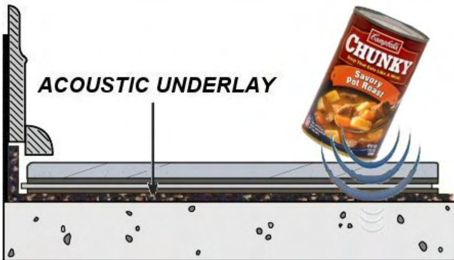
Under the IIC/STC rating system, the higher the number rating assigned to sound insulation, the better. In other words; rooms become increasingly quiet as the number increases. In contrast, a poorly insulated wood frame sub floor assembly may rate as low as IIC/STC-35 dB (decibels) or less. Most Condo Associations and Municipalities have adopted the International Building Code or Universal Building Code minimum rating of IIC-STC-50. Some luxury properties and
