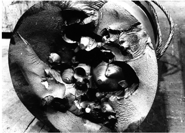
Illustration 43: Hydrogen initiated breakage of a forged back-up roll
