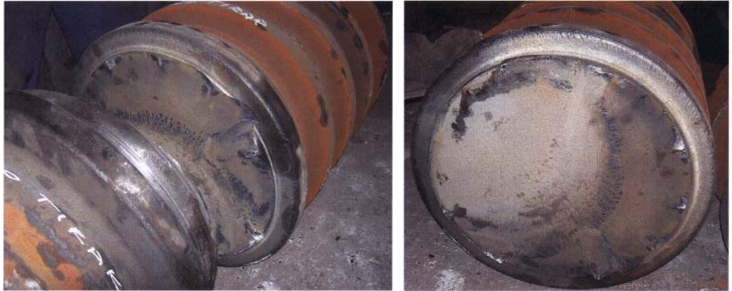
Illustration 38: :Fatigue failure/breakage of a section mill roll.
