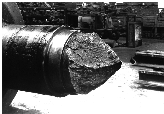
Illustration 37: Neck failure from drive end torque
