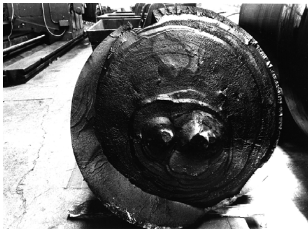
Illustration 44: Hydrogen initiated breakage of a cast back-up roll
