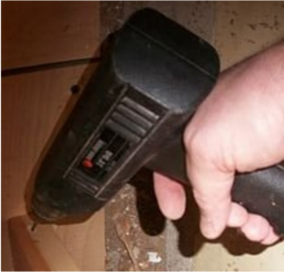
Figure.2.2. Drills can also be used at an angle to join two boards
