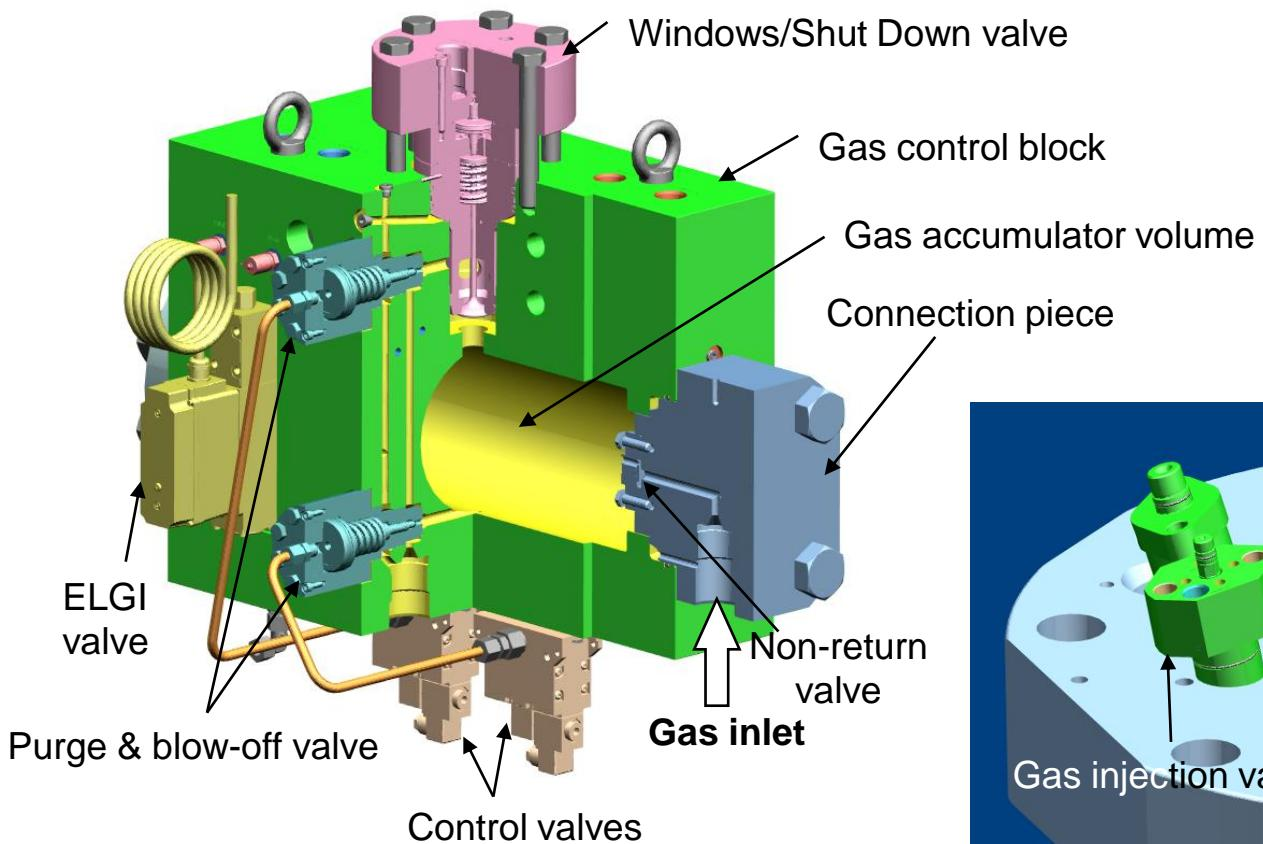
Same design used for gas test rig in Copenhagen and on our test engine Q4, 2010
