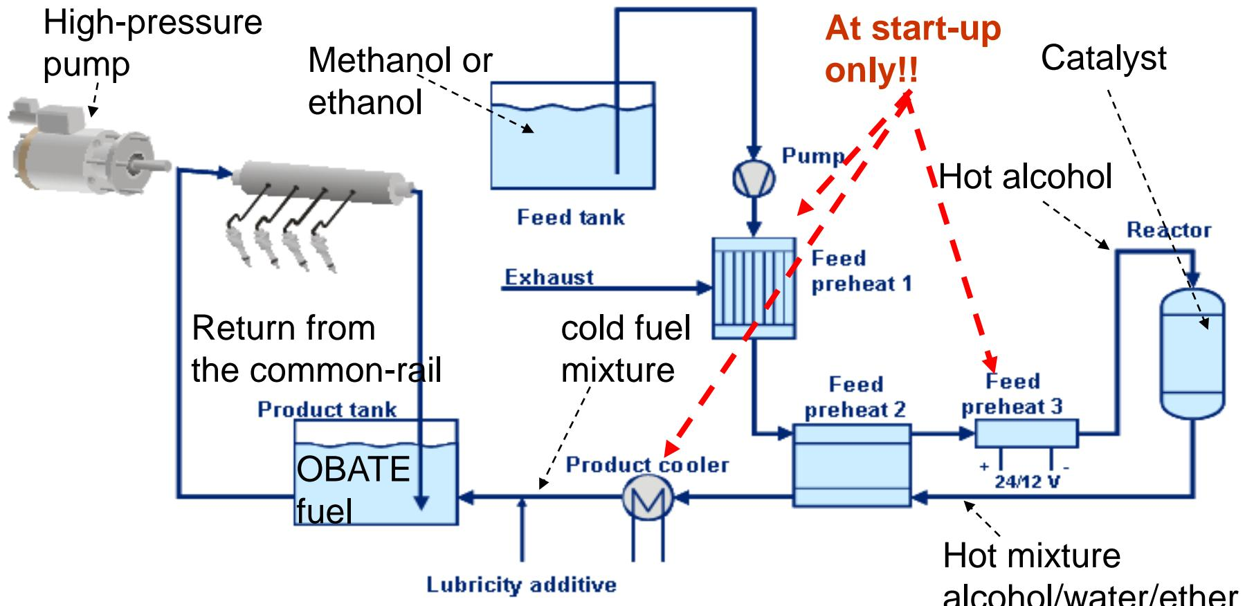
The process is auto-thermal: the OBATE fuel has the same heating value than the original fuel!!
