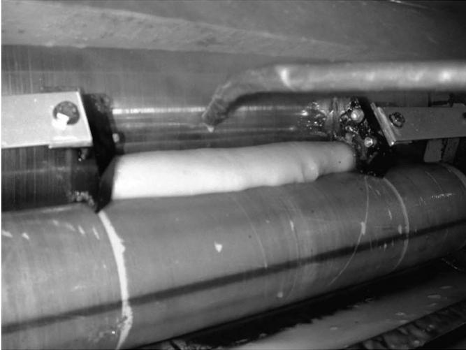
**FIGURE 12.12** A detailed view of the “bourbier” between the drum and its feed roller (pilot plant, AgroParisTech, Massy).
