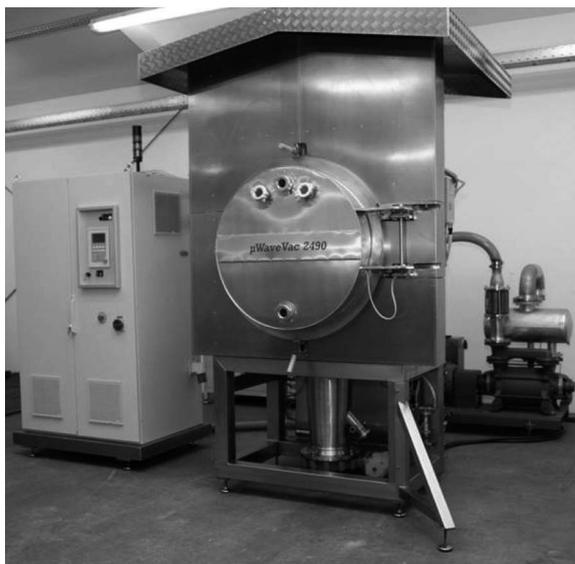
**FIGURE 13.3** Batch MW–vacuum dryer. (From Püschner Microwave Power Systems, <http://www.pueschner.com>, 2007. With permission.)
