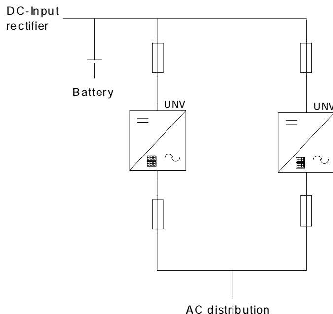
Inverter UNV-F converts input side DC voltage to stable sinewave output voltage.
